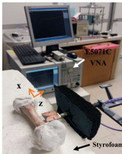
FIGURE 9: Details of the configuration of one of the microwave imaging systems.
