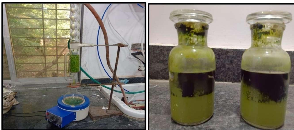
Fig.No.3 Soxhlet assembly and crude extract of Tinospora cordifolia
