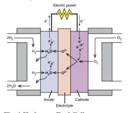
Fig. 1 Hydrogen Fuel Cell
