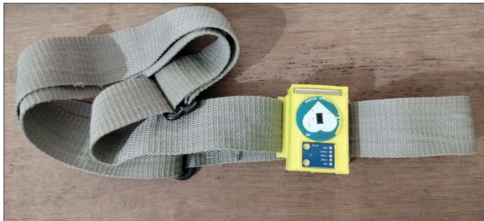
Figure 2. Smart Neck Collar equipped with sensors
