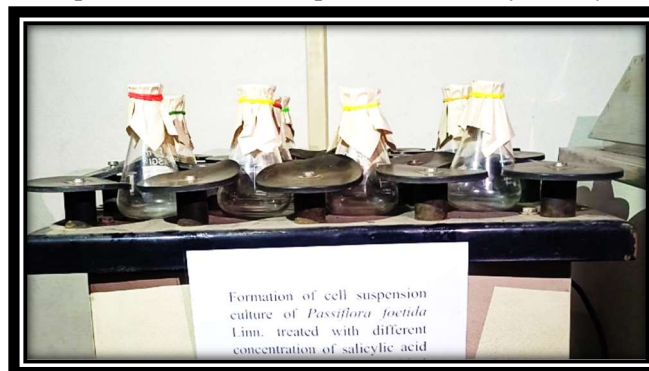
Figure:5 Forming cell suspension culture of Passiflorafoetida Linn. treated with various concentration of salicylic acid (orbital shaker).
