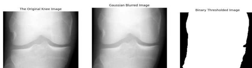
Figure 3– The ROI extraction process – Original image, Gaussian Blurred image (kernel – 3x3), and the Binary thresholded image (threshold – 80)
