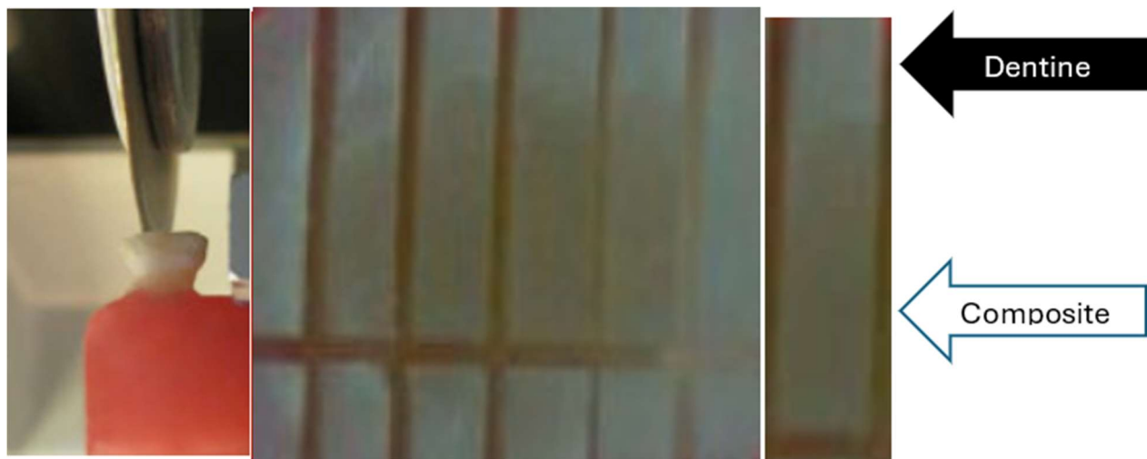
Figure (5): A photograph showing preparing a specimen to be measured by the Micro-tensile bond strength.
