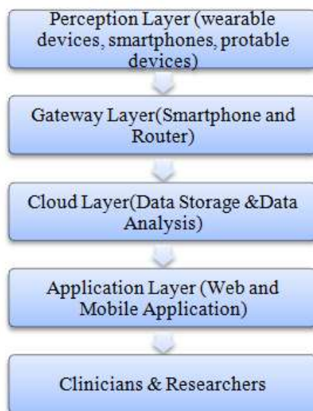
Figure 1 Block Diagram IoT based Fetal Health care System
