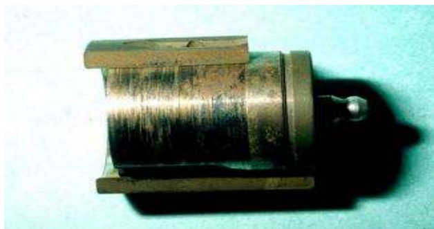
Figure 02 Corrosion friction of a piece in steel [3]
