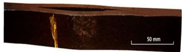
Figure 22 Blistering related has an overprotection cathodic of a pipeline oil. [3]
